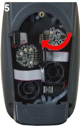
5 Insertion of a new sensor then rotation of the sensor
