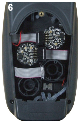
6 Connection of the sensor ribbon cable
